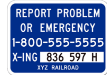
Emergency Notification Systems sign
