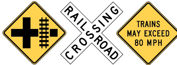
Crossbuck and railroad signs
