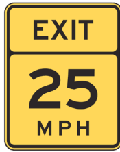
Off Ramp Advisory Speed sign
